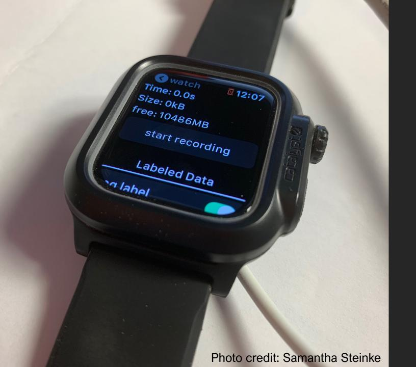
Apple watch used as IMU for trials with SensorLog recording application.
