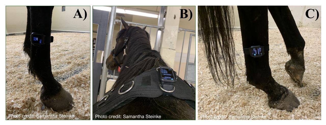
The locations in which the Apple watch was placed for movement analysis trials. A) right forelimb B) withers attached to surcingle C) right hindlimb.
